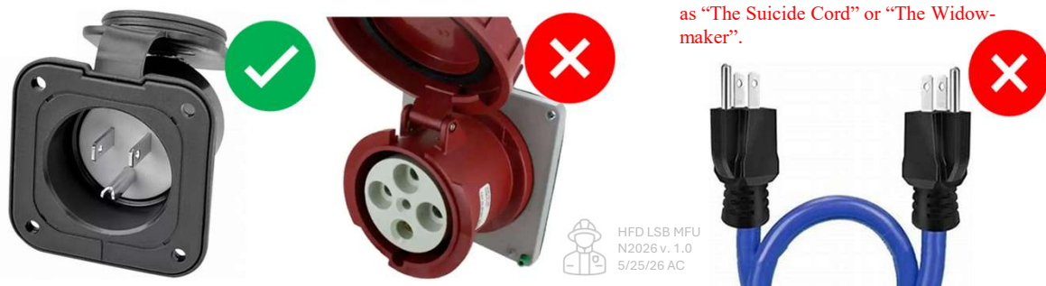
Figure 6. Your service-entry power supply shall have a male inlet, secured to the Food truck, in a weather rated casing or a direct connection to the breaker box. Never use a double male connection.
